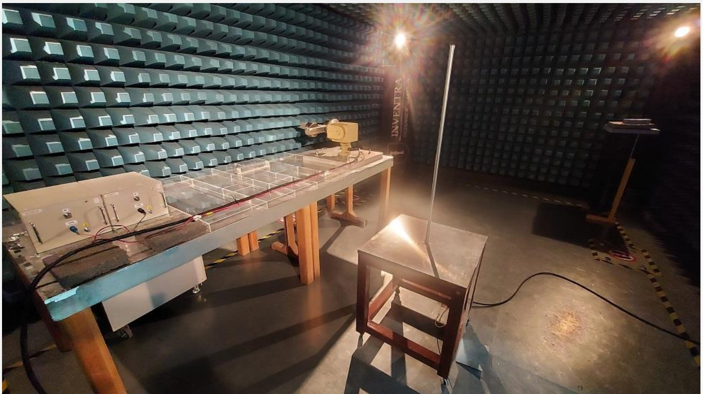
RE102 and CE102 Test Setups
