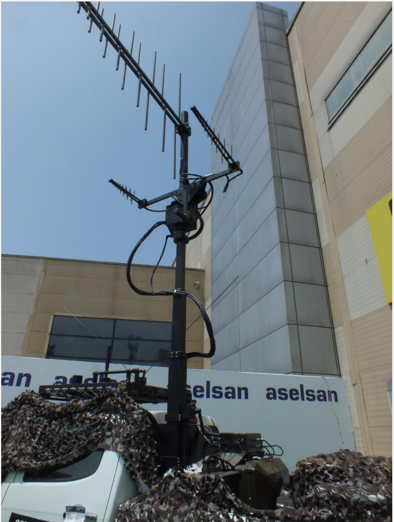
The PED10 Positioner and MMS10 Mast Systems carry payloads with a significantly offset center of gravity on a vehicle platform at the IDEF International Defense Industry Fair.
